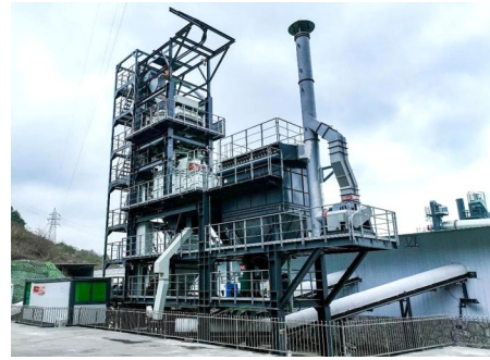
图1 RAP精细化处理与原生拌和系统 Figure 1 Refined treatment of RAP and primary mixing system
