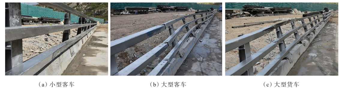
图 14 碰撞后护栏的形态 Figure 14 Form of guardrail after collision
