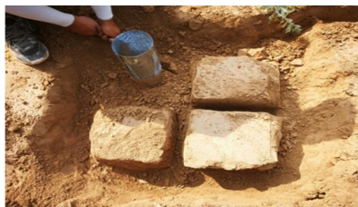
图1 原状样取土现场图片 Figure 1 Pictures of on-site extraction of soil in its original state
