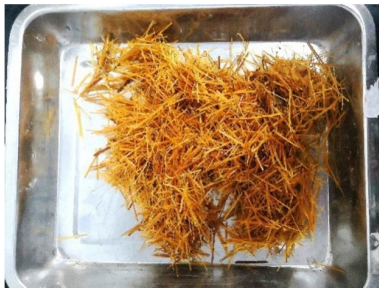
图4 经碱处理后的竹纤维 Figure 4 Bamboo fiber treated with alkali
